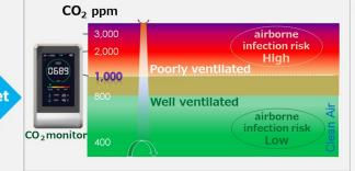
CO<sub>2</sub> below 1,000ppm: Ventilation is sufficient.
